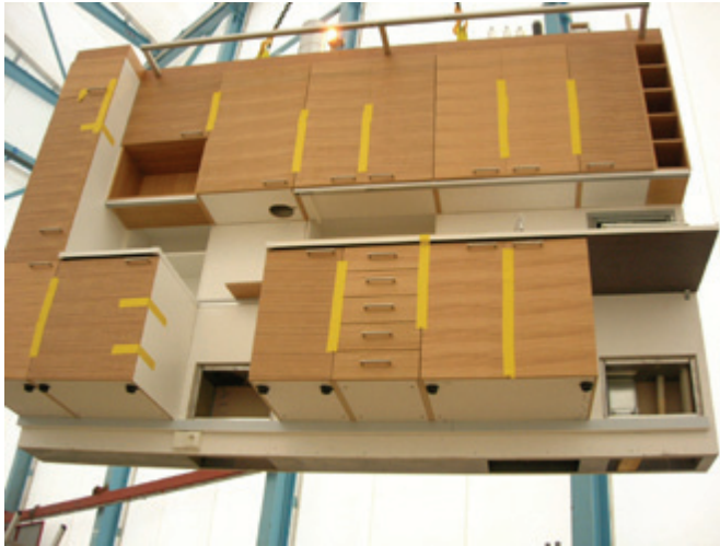
Fig. 10. NCC Komplet wall assembly in on site assembly hall
