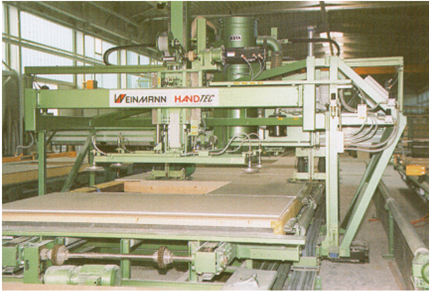
Fig. 5. Multifunctional robotic wooden wall production unit
