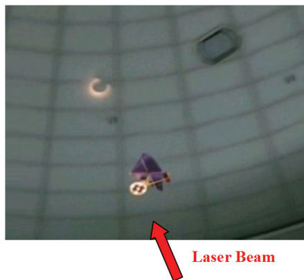
Fig. 7. Flying kite plane under the auto-tracking (The solar panel is irradiated by the laser light with its shade on the ceiling)
