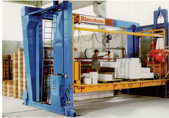
Fig. 2. Factory based mobile semi automated masonry wall production unit including automated mortar distribution
