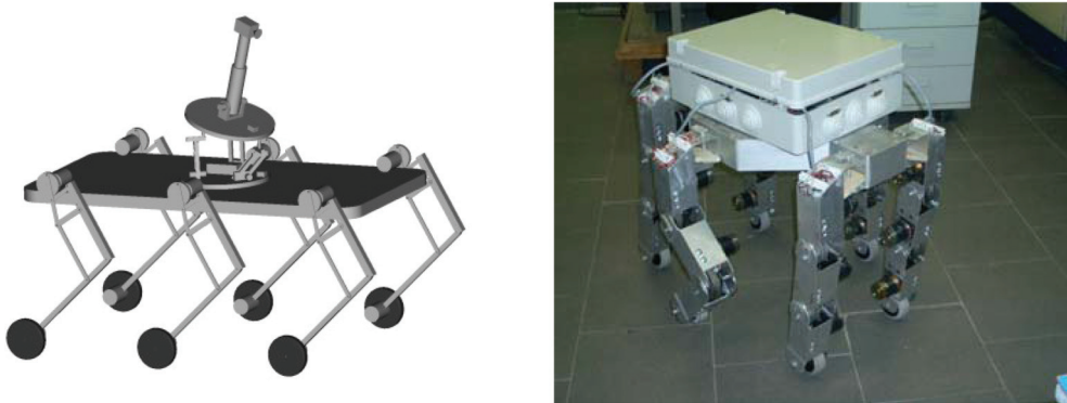
Fig. 15. The Cassino hexapod robot for Survey activity as a general kinematic scheme and a built prototype.
