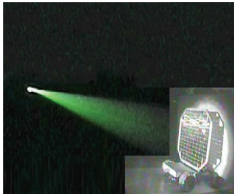
Fig. 2. 1 km laser energy transmission to a model lunar rover has successfully been done
