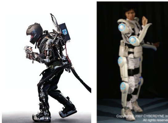
(b) Exoskeleton System for Whole Body Support ('XOS' of SARCOS and 'HAL' of Cyberdyne Inc.)
